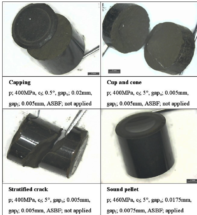
Fig. 1. Visuals of the green pellets for the Ce–MOX with the compacting parameters: p (compacting pressure), c_f (chamfer angle in the outlet of a die), gap_u (radial gap between the upper punch and die), gap_l (radial gap between the lower punch and die), and ASBF (anti-spring back force on the upper punch).
